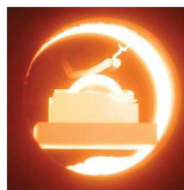
Fig. 3. Silicon droplet on a quasi-single crystal substrate (at a holding time of 1 min)
