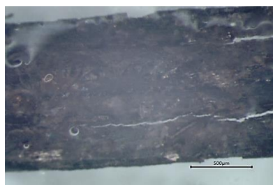
Fig. 7. Corrosion cleavage of alloy (Al_{74}Cu_{16}Mg_{10})_{99}Zn-a after 360 h in NaCl at 50 °C
