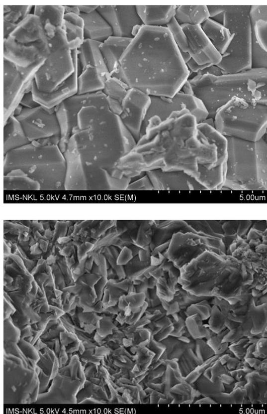
Fig. 2. SEM image of Tan-rai AH (top) and the one after grinding for 18 h, and cleaning with acetic acid (bottom)
