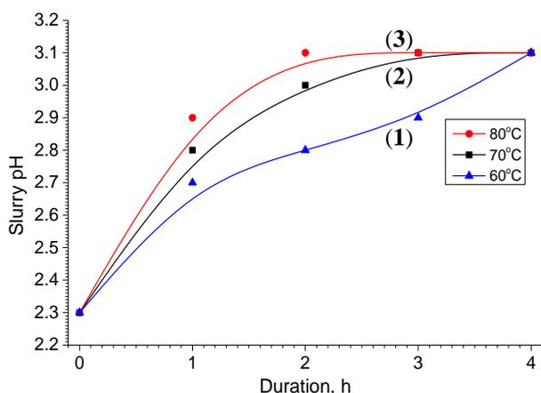
Fig. 3. The pH change in the suspension during mixing of the ground AH with 1 N acetic solution at the temperature of 60 °C (1), 70 °C (2) and 80 °C (3)
