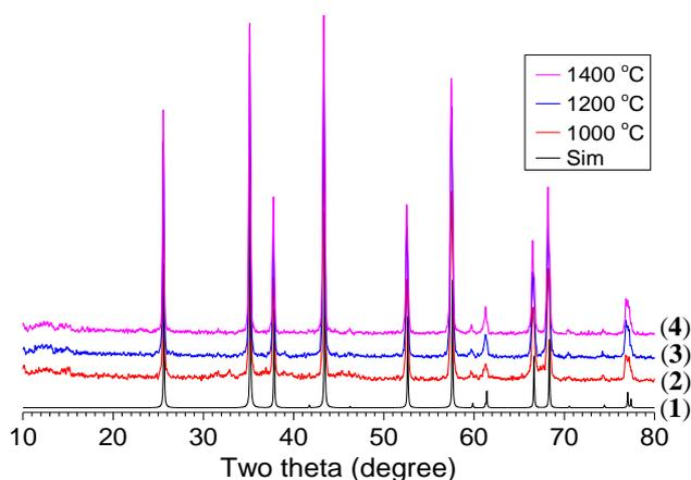
Fig. 4. The XRD patterns of thermal decomposition products when the samples are heated for 2 h at 1000 °C (2), 1200 °C (3), 1400 °C (4) and the simulated one (1) of  $\alpha$ -alumina based on data from JCPDS No. 83-2080
