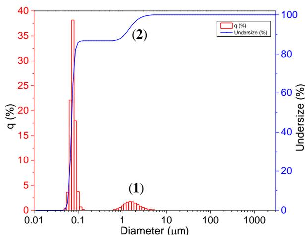
Fig. 5. The particle size distribution (1) and cumulative undersize (2) of the prepared  $\alpha$ -alumina after heating at 1400  $^\circ\text{C}$
