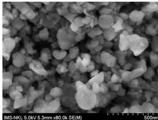
Fig. 6. SEM image of  $\alpha$ -alumina prepared from AACH when heated at 1400  $^\circ\text{C}$
