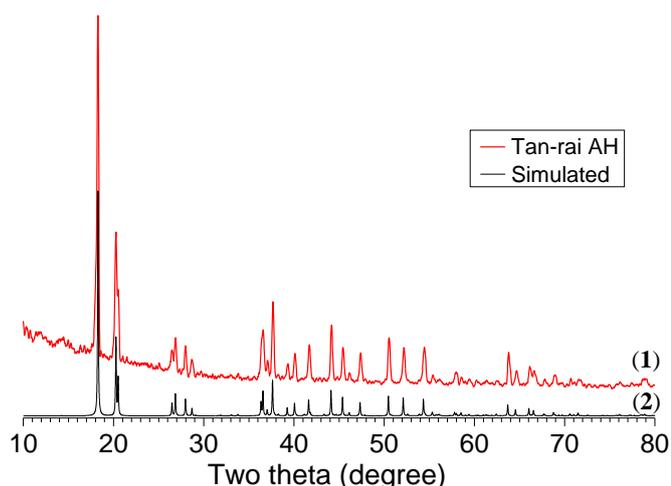
Fig. 1: The XRD pattern of Tan-rai AH (1) and the simulated one (2) based on data from JCPDS No. 03-0145 for the gibbsite phase
