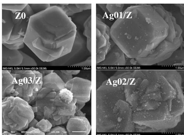
Fig. 2. SEM images of Z0, Ag01/Z, Ag02/Z, Ag03/Z
