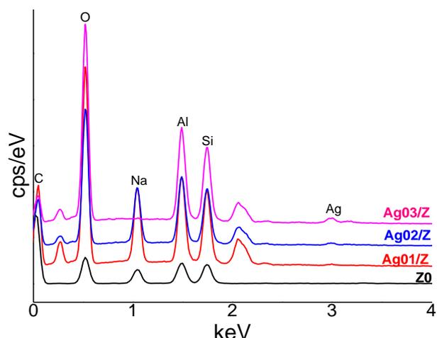
Fig. 1. Energy-dispersive X-ray spectroscopies of Z0, Ag01/Z, Ag02/Z, Ag03/Z samples
