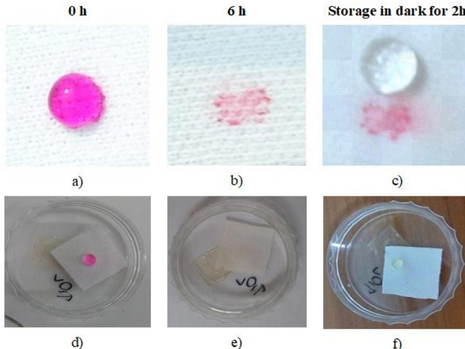
Fig. 4. Photodegradation of Rhodamine B in TiO<sub>2</sub>/PET (a, b, c); Ag-TiO<sub>2</sub>/PET (d, e, f) under visible light in solid state after 6 h
