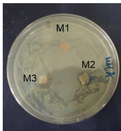
Fig. 3. Antibacterial effect of PET blank (M1), PET coated by TiO<sub>2</sub> (M2) and PET coated by Ag-TiO<sub>2</sub> (M3).
