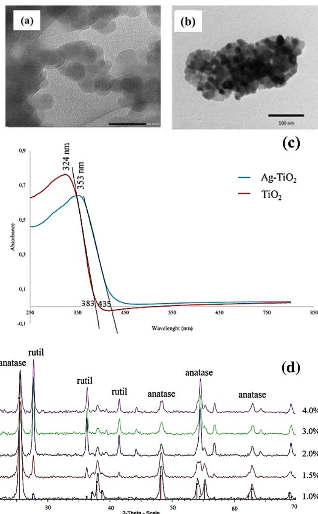
Fig. 1. Characterization of TiO<sub>2</sub> and Ag-TiO<sub>2</sub> nanoparticles: TEM images of TiO<sub>2</sub> (a), and Ag-TiO<sub>2</sub> (b) nanoparticles; UV-Vis spectra of Ag-TiO<sub>2</sub> and TiO<sub>2</sub> nanoparticles (c) and XRD spectra of Ag-TiO<sub>2</sub> nanocomposite in different ratios Ag<sup>+</sup>/Ti<sup>4+</sup> (d).
