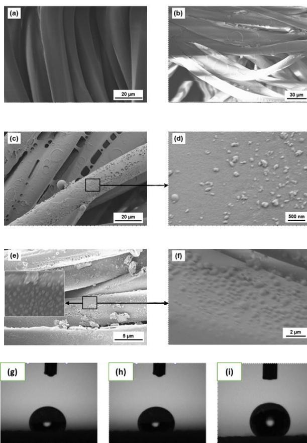
Fig. 2. SEM surface images of untreated PET fabric (a), treated PET fabric with binder (b), PET fabrics coated by TiO<sub>2</sub> nanoparticles with binder (c, d) and PET fabrics coated by Ag-TiO<sub>2</sub> nanoparticles with binder (e, f) and static water contact angle on the surface of fabric by binder (g) coated with TiO<sub>2</sub> (h) and Ag-TiO<sub>2</sub> nanoparticles (i).
