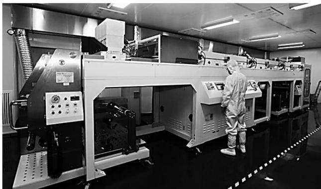
Fig. 1. Film printing equipment by roll-to-roll mode
