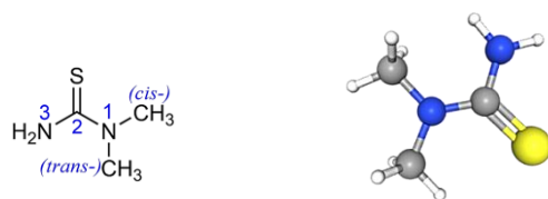
Fig. 1. Structure of the N,N -dimethyl-2-thiourea (1,1-DMTU) molecule with nitrogen and carbonyl C atoms numbered (3D-version: B3LYP/6-31G*, Gaussian 09-D.01)
